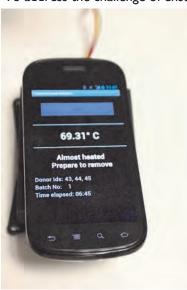
in homes and resource-limited health care facilities. PATH is advancing a safety management system based on a platform called FoneAstra. FoneAstra is a realtime temperature monitoring device and remote data recording tool. This system leverages mobile phones to precisely monitor flash-heat pasteurization of
